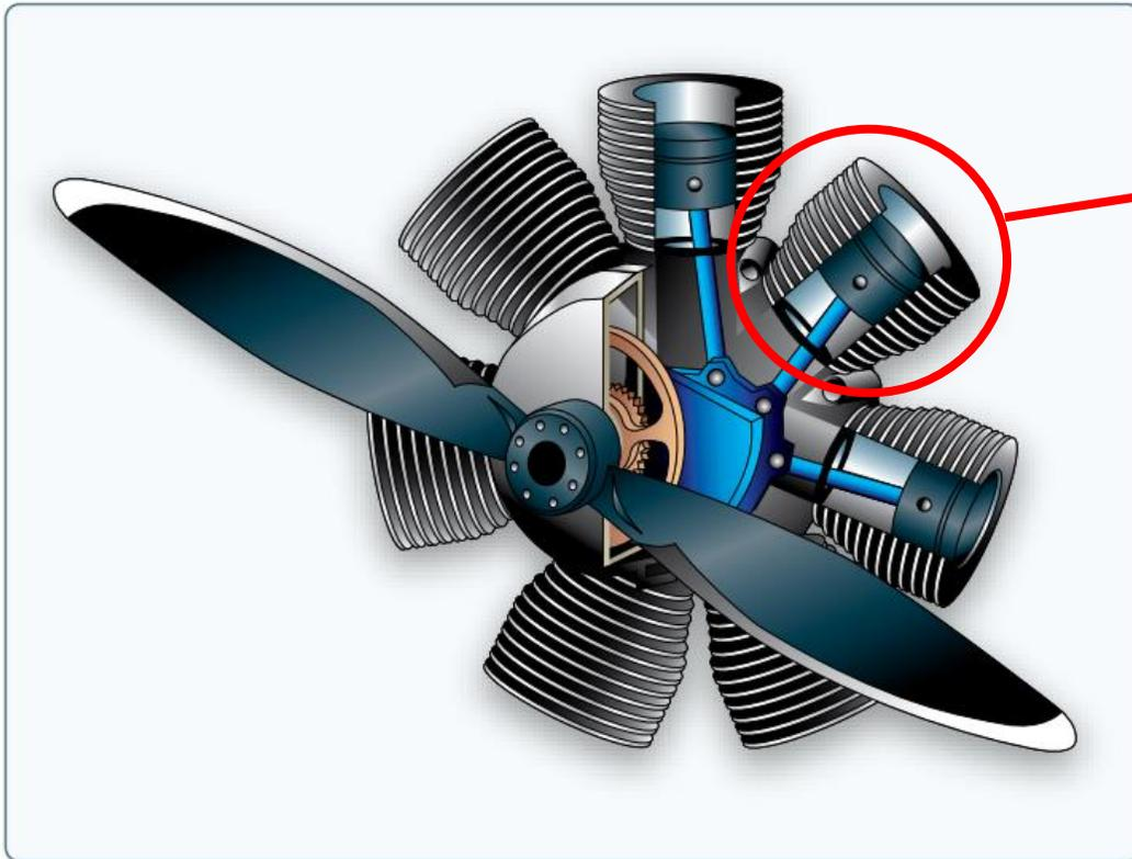
Figure 7-1. Radial engine.
