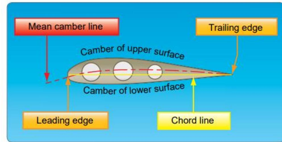
**Figure 4-5.** Typical airfoil section.
