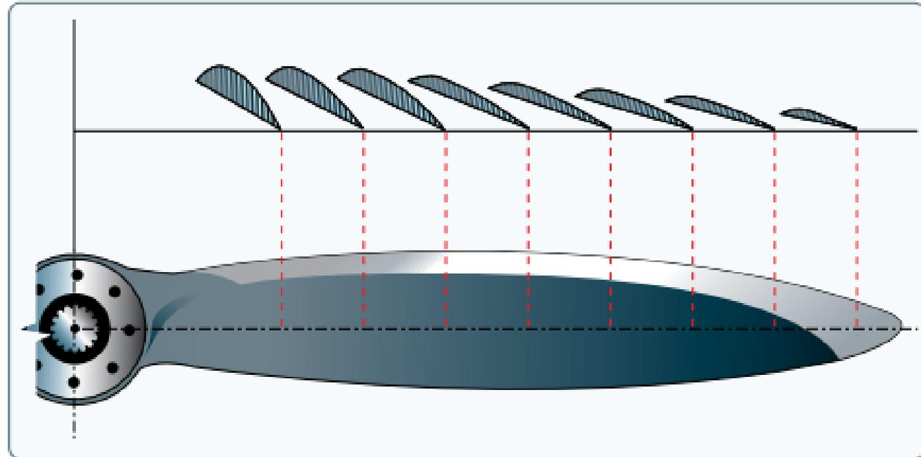
**Figure 5-43.** *Airfoil sections of propeller blade.*
