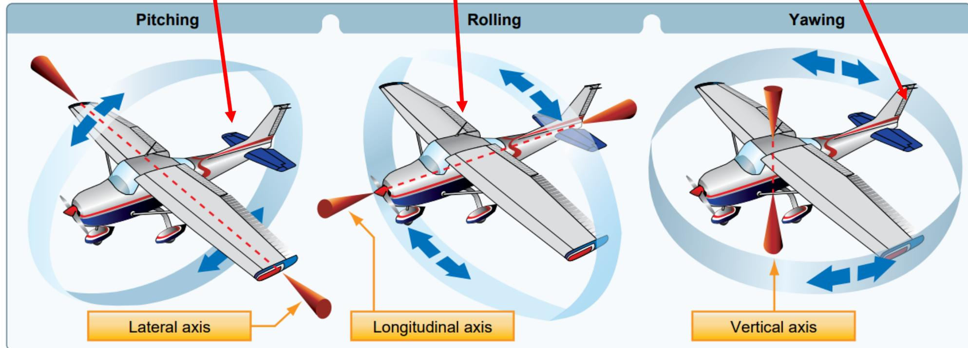
Figure 5-18. Axes of an airplane.
