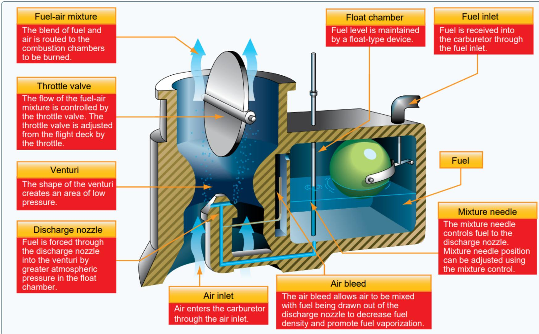
Figure 7-10. *Float-type carburetor.*
