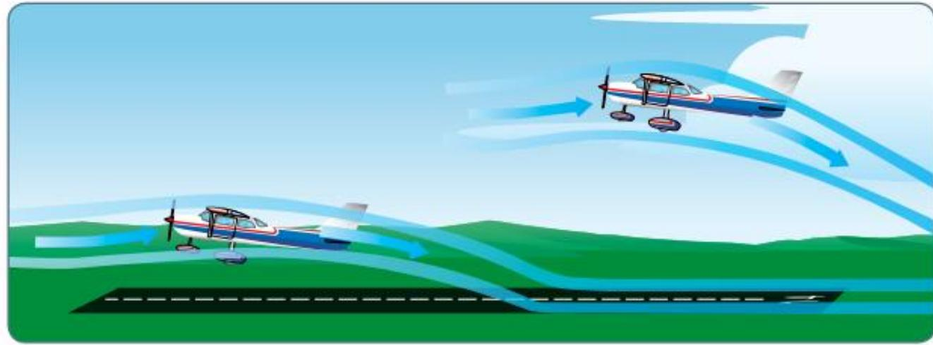
**Figure 5-16.** *Ground effect changes airflow.*
