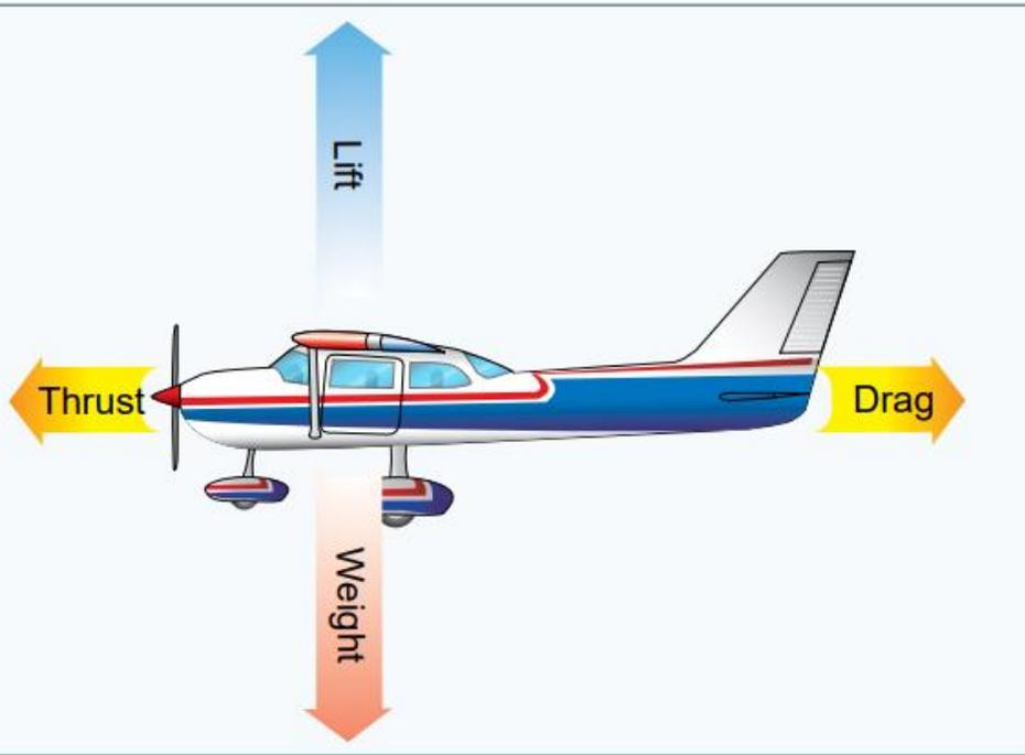
**Figure 5-1.** *Relationship of forces acting on an aircraft.*
