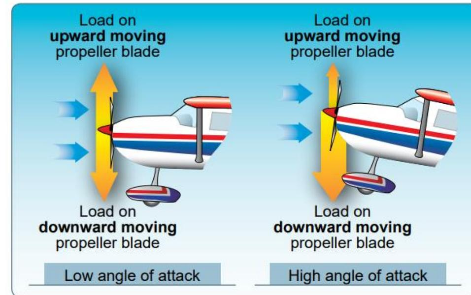
Figure 5-51. Asymmetrical loading of propeller (P-factor).
