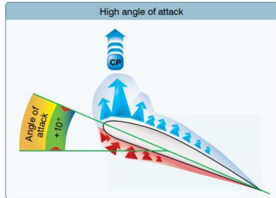
**Figure 4-7.** Pressure distribution on an airfoil and CP changes with AOA.
