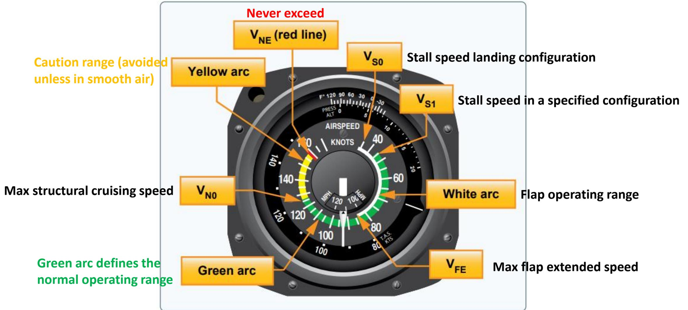
Figure 8-8. Single engine airspeed indicator (ASI).
