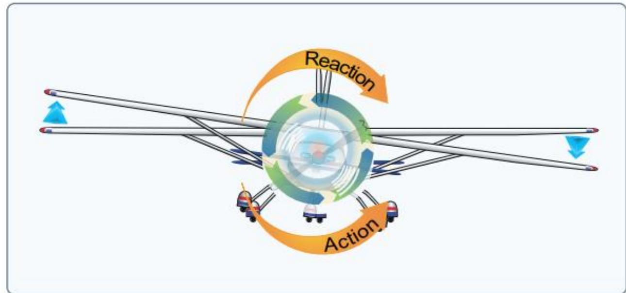
Figure 5-47. *Torque reaction.*
