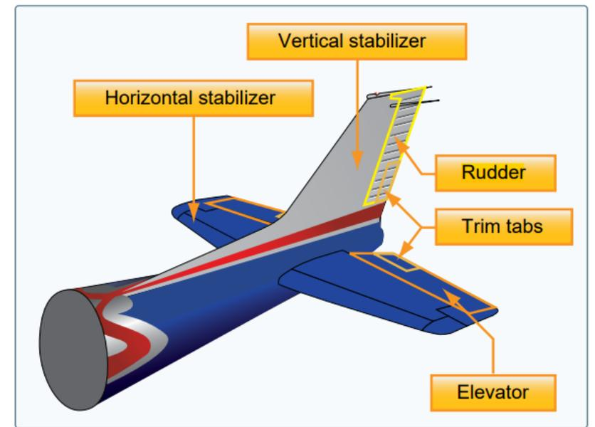
Figure 3-10. Empennage components.
