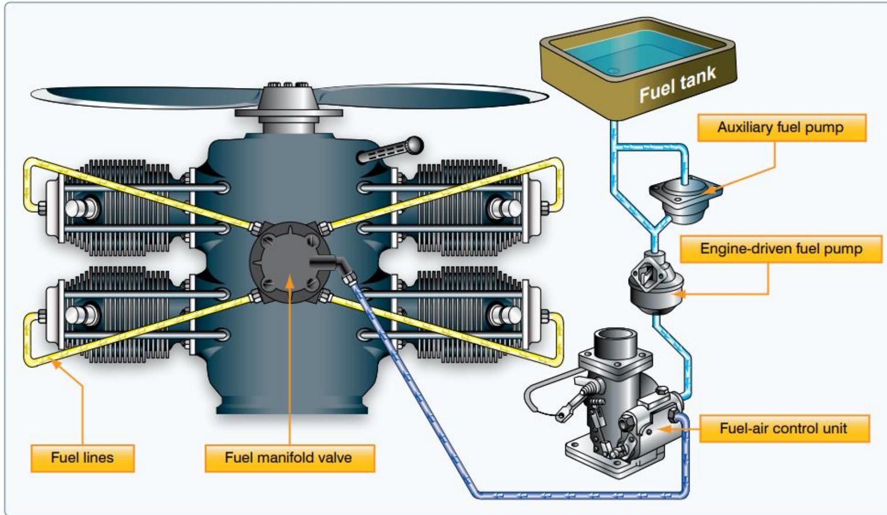
Figure 7-13. Fuel injection system.
