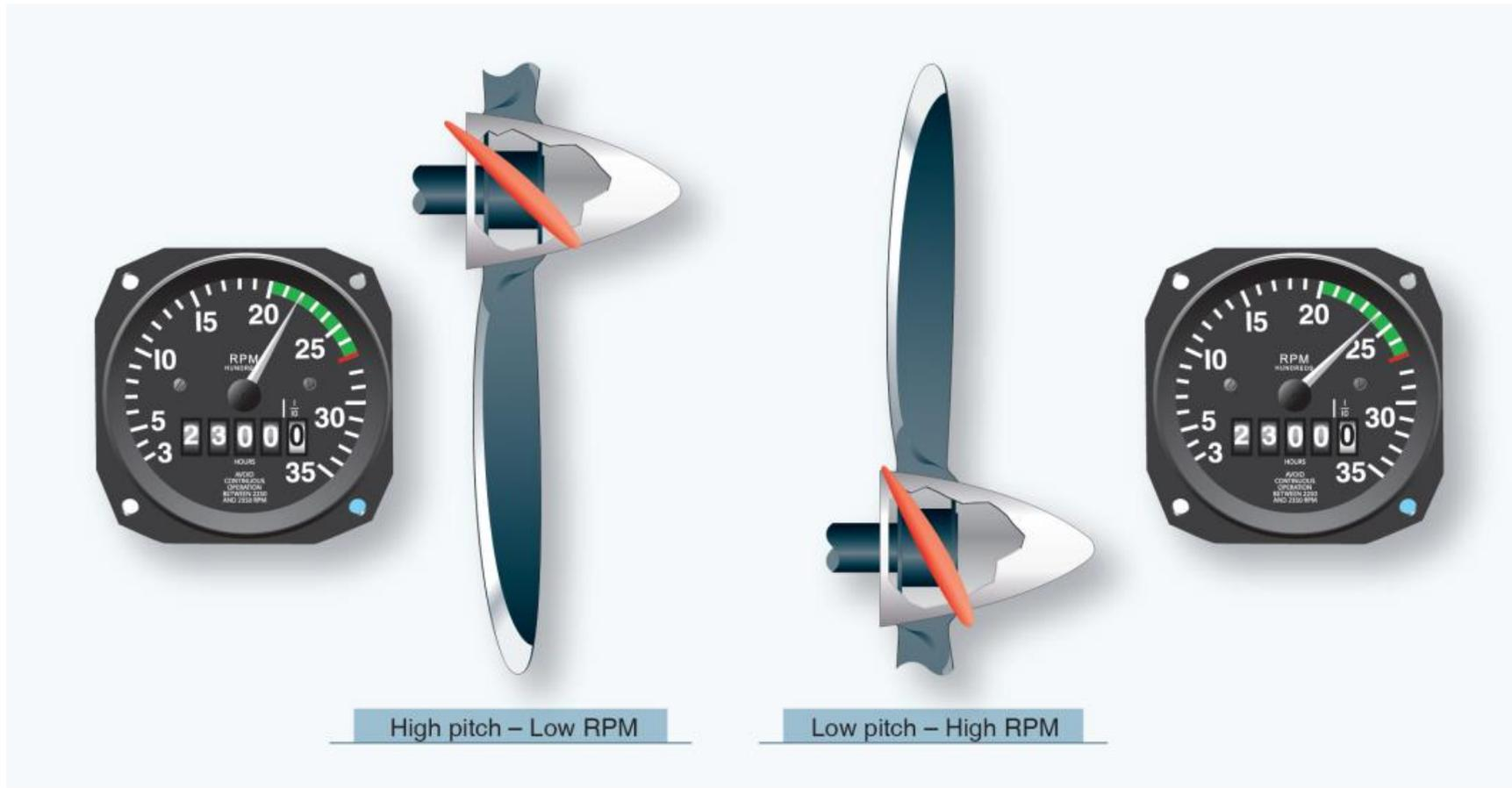
Figure 12-6. Controllable-pitch propeller pitch angles.
