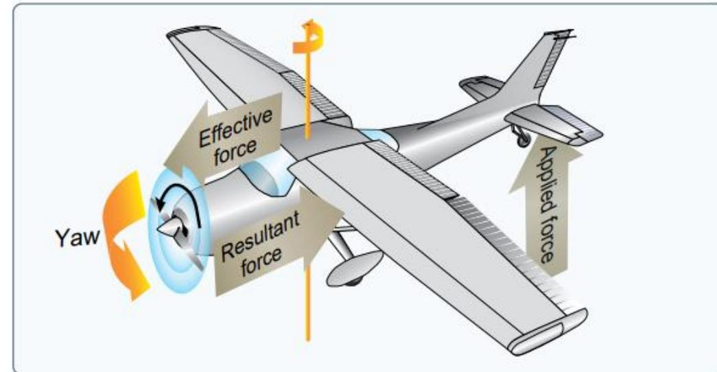
**Figure 5-50.** Raising tail produces gyroscopic precession.
