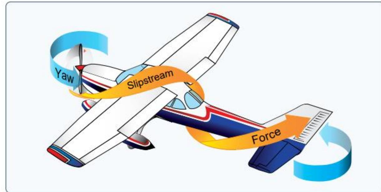
**Figure 5-48.** *Corkscrewing slipstream.*
