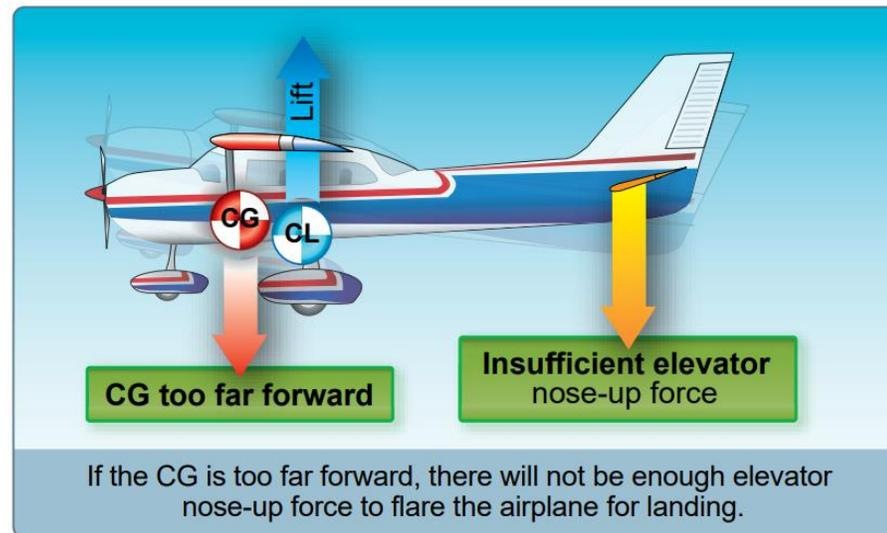
Figure 3-3. Center of gravity (CG).
